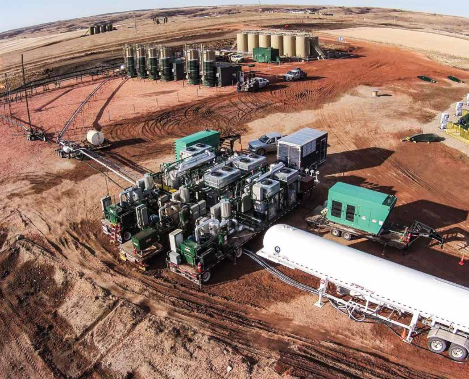
A Berg-GTUIT mobile refrigeration unit captures natural gas and separates out the valuable liquid hydrocarbons in North Dakota's Bakken shale oilfield.
