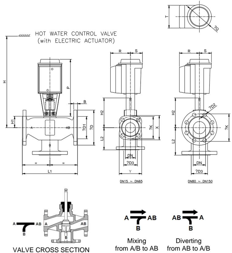
Hot Water Control Valve Dimensions (unit : mm)
